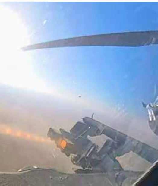
Opposite page left: An AGM-114L Longbow Hellfire missile launches from the Surface-To-Surface Missile Module (SSMM) aboard Independence-variant Littoral Combat Ship USS Montgomery (LCS 8). The missile exercise was the first proof of concept launch of the Longbow Hellfire missile against a land-based target. LCS is a fast, agile, mission-focused platform designed to operate in near-shore environments, winning against 21st-century coastal threats. LCS is capable of supporting forward presence, maritime security, sea control, and deterrence.
